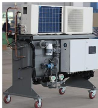
Figure 2 Absorption Regenerator
