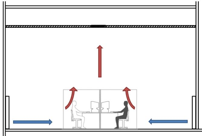
Figure 1 Displacement Air Distribution
