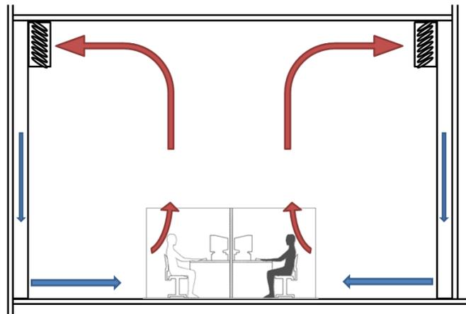
Figure 3 Passive Thermosiphon Beams
