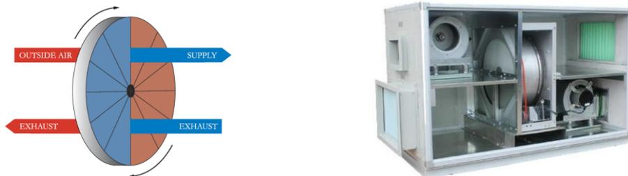
Figure 2 Mechanics of an enthalpy wheel.
