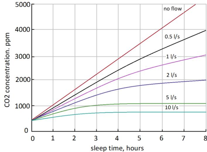
Fig. 1 CO<sub>2</sub> build up during sleep for a bed room with volume of 21m<sup>3</sup>
