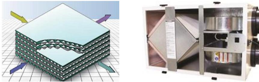
Figure 3 Configuration of a fixed-plate heat exchanger.
