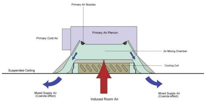
ABM supply cooling/heating to the space through the following mechanism:
